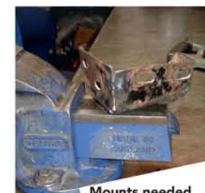
Mounts needed rewelding to finish.
