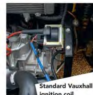
Vauxhall XE twin cam with Yamaha bike carburetors.
