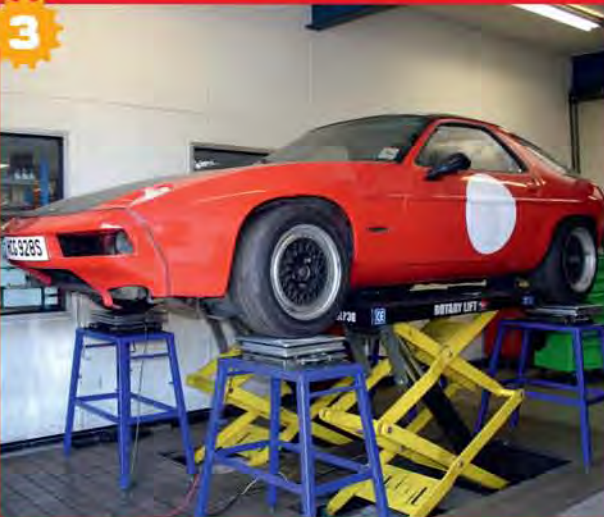
3 Sitting on the scales the total weight is down to 1157kg including the cage and safety equipment (from 1600kg). The corners were Fronts R 333, L 326, Rears R 237, L 261.
