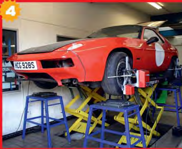
4 As the rear suspension arms had been removed the geometry had to be re set. The rear camber was set up to one degree negative with ten minutes toe-in.
