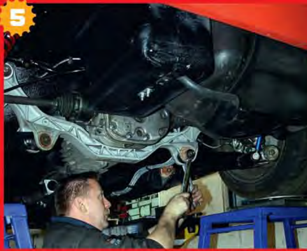
5 With the settings within tolerance the eccentric adjusters were locked off. Last time we tried to adjust the rear suspension it was seized but now it's rebuilt this was easy.
