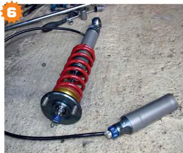
6 Here's one of the new shocks with its separate canister. This has the bump adjusters on it, so mounting it inside the car makes adjustment much easier than if it were on the shock.
