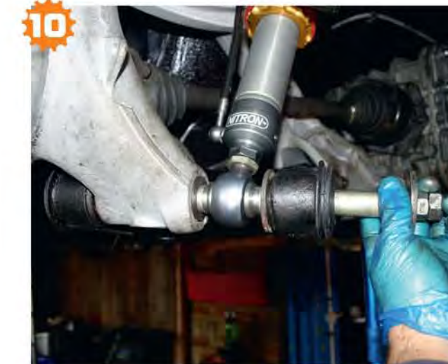
10 The lower mount is a whopping 22mm shaft that goes through the lower wishbone twice, the rear upright and the shock absorber. Fitting the bushes at the same time was fun.
