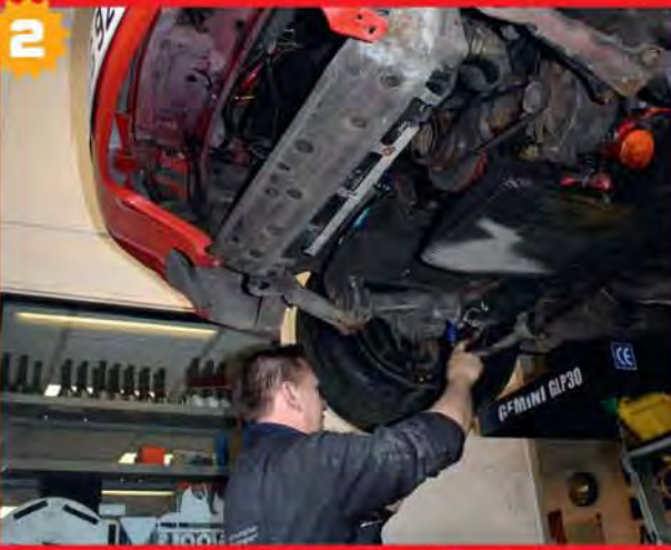
2 First step was to release the drop links. The theory is set the shocks to get the right corner weights then adjust the drop links so they are not under tension and reconnect them last.
