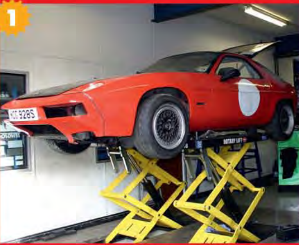
1 We took the car along to Troy at Northampton Motorsport as he's seen the car before. With adjustable platforms on all four shocks we could get the ride height spot on.
