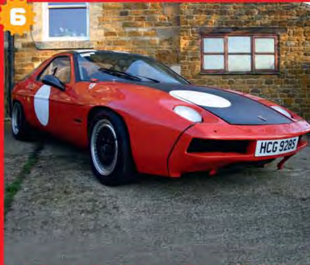
6 With the car back on the ground we could see the new lower ride height for the first time. The tyres are now much nearer the arches but the ride is much harder so they may be okay.
