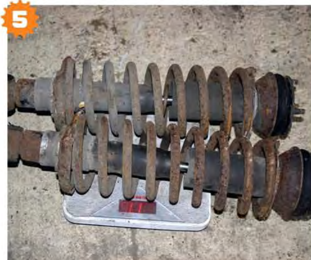
5 Here's the proof of how much the original shocks weigh. In total the four old shocks weighed 35kg whereas the new set-up including remote reservoirs is just 16kg. Go figure.
