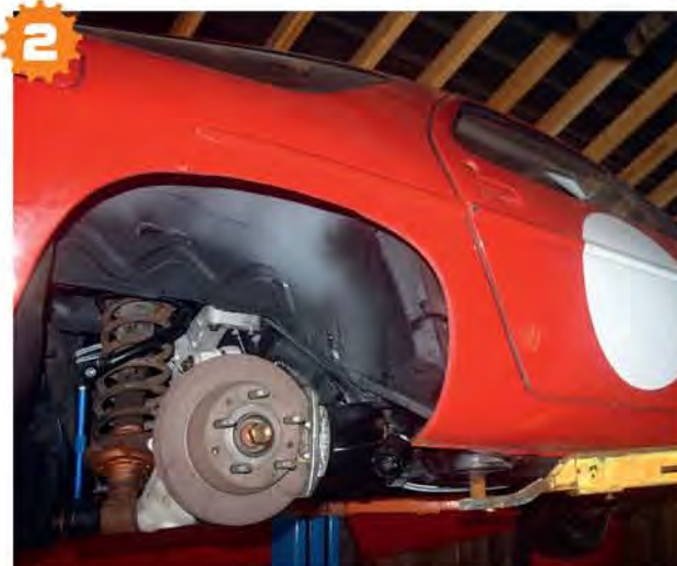
2 We'd recently had the rear shock absorbers off the car so we weren't expecting any problems. The top mount bolts through into the boot, the bottom mount is a large 22mm bolt.
