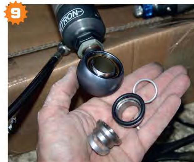
9 The bottom mount of the rear shock needed some spacers to be made up. The O-ring seals the spherical joint while the other two other bushes space out the lower bolt.
