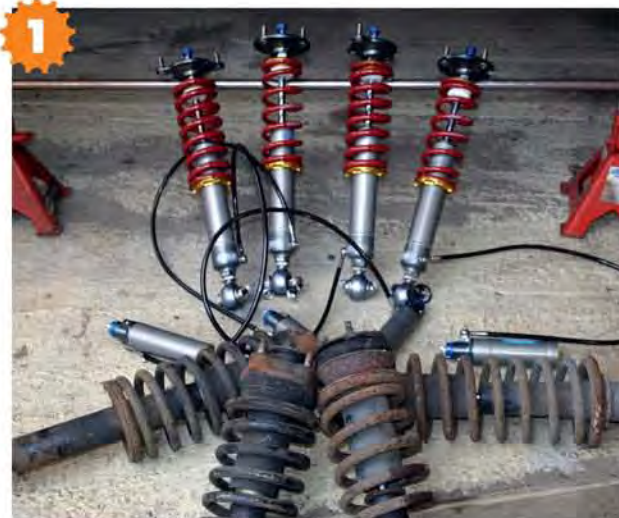
1 The first thing to note about the Nitron remote reservoir kit is how small and light it is compared with the original Porsche suspension. The reduced size helps a lot when fitting the fronts.
