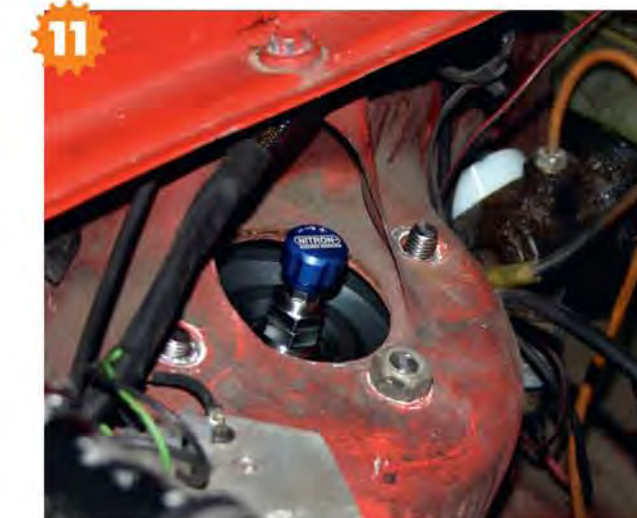
11 At the front under the bonnet the nuts were much easier. The top mount has room for the adjuster to fit through and the nuts were easy to get on with a socket and ratchet.
