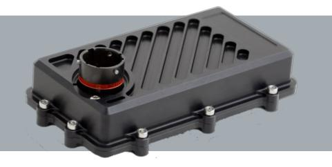
Life Racing's direct injector driver is a compact unit capable of driving four fuel injectors at a high voltage, thus catering for the requirements of high-pressure solenoid injectors. The unit generates the complex waveforms required to activate the injectors. The injectors are switched on via pulses from the host ECU.
