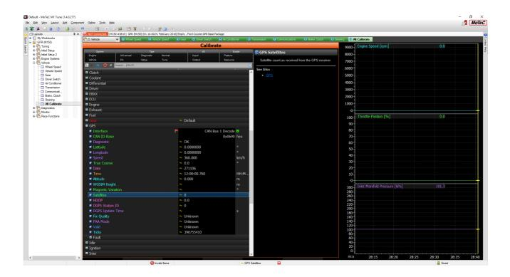
The Gyro/IMU Information needs to come via the Bosch MM5 protocol. Select Bosch in All Calibrate and set the CAD ID Messages as below
