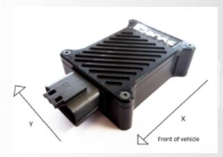
In applications where heavy vibrations are present due to solid engine mounts etc, it is advised to mount the GPS using some rubber washers to absorb some of the vibrations.
