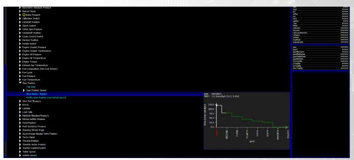
Flat Shifting - When the Clutch is pressed on it will send a GearCut Request into the ECU for Flat Shifting. This is Setup in Gearcut - Open Loop
