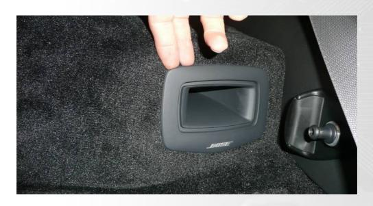
4.) Lift the carpet to reveal the Ecu Cradle which is removed by 3 x M6 nuts
