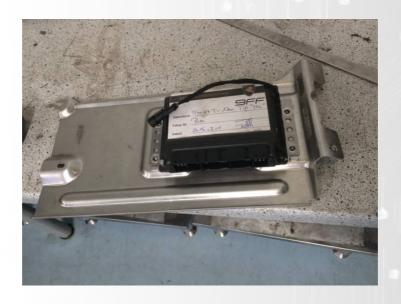
6.) Next Mount the Syvecs PNP ECU onto the Factory bracket, it will bolt straight into the OEM Location
