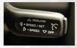
Pushing the stalk button down towards the Off Symbol and holding is used to go back down the Calibration switch positions.
