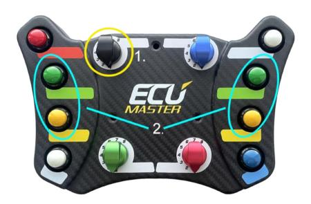
When the rotary switch indicates the desired power level, confirm the change by pressing the 4 buttons highlighted in **blue** for a **minimum of 3 seconds**. Confirmation of the power change will be reflected in the **Tx power lvl** channel in the channels window of the Light Client. An example of changing the power from the highest to the lowest is shown in the image below:
