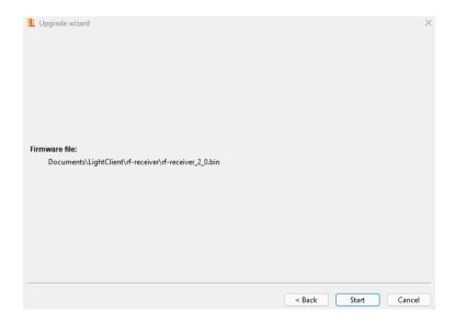
Next, press the "Start" button to upgrade the firmware. Crucially, avoid turning off your PC or interrupting power to the device during the upgrade.
