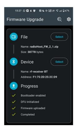
Confirmation of the successful upgrade procedure will be the information about the firmware version in the Channels window *Receiver radio FW* of the Light Client and the change of the **Receiver State** parameter from **Bootloader** to **Active**. The CAN diagnostic frame must be enabled to see the *Receiver radio FW* channel.
