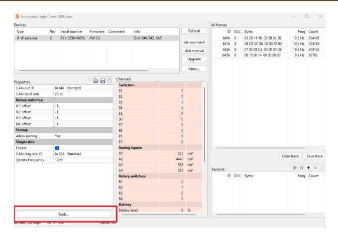
Once you select "Go to receiver bootloader" in the Light Client application, the Wireless Receiver enters bootloader mode. To **confirm successful entry**, check the **Receiver state** channel within the application.
