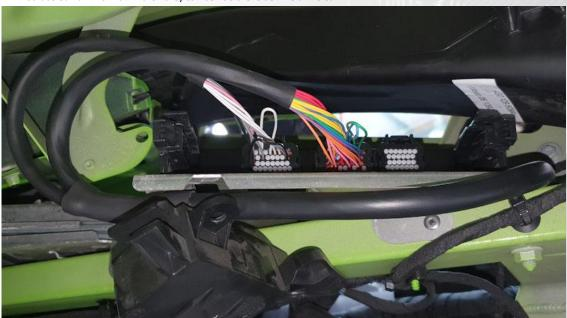
7.) Plug in the GDI Fuel Pump wires to each pump. Pay attention to the Bank Allocation labels
