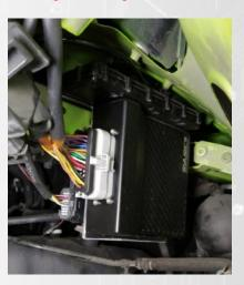
6.) Fit the Syvecs Interface boxes in the mounts which are for the OEM Ecu then route the loom as shown below - If the interface boxes are not labeled Bank1 or Bank2 then they can be fit either side... i.e universal
