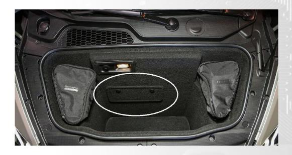
2.) Remove the Engine bay covers shown below by turning the fasteners anti clockwise which are marked in Red
