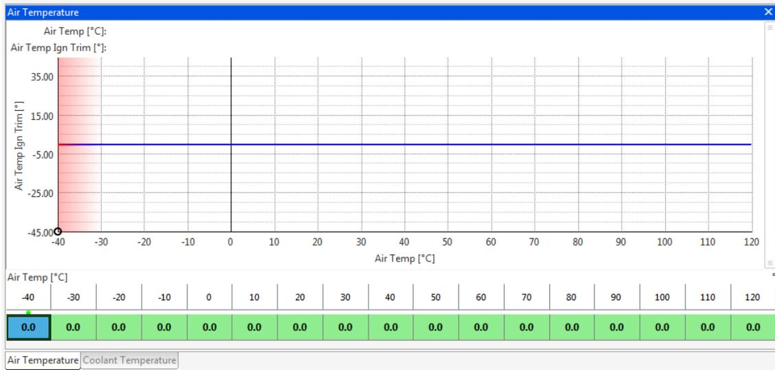
Ignition can be trimmed based upon air inlet temperature. This is only used for extremes of temperature. This is described by the **Air Temp Ign Trim table**.
