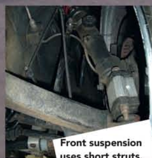
Dampers are two-way adjustable.
