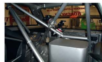
Cage picks up suspension mounts.
