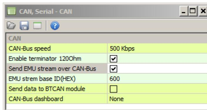
It is critical that you enable “Send EMU stream over CAN-Bus”. This activates the EMU standard CAN stream with critical ECU parameters like RPM, CLT, state of coolant fan, fuel pump, etc. More information about the EMU standard stream can be found in help menus of the EMU software. Another important parameter is EMU stream base ID. In this example the value is 0x600 and is the default CAN stream ID.
