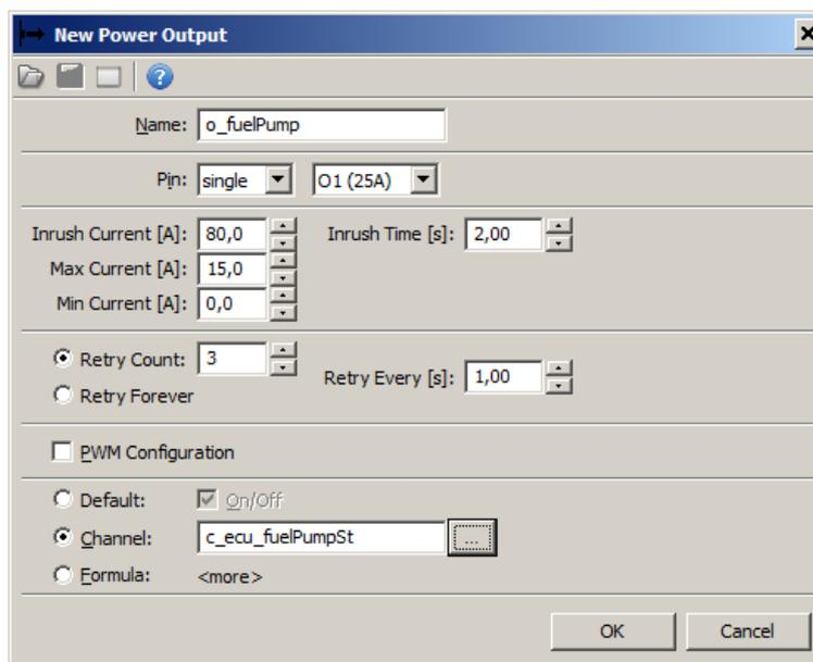
Set output name and configure the currents. As you can see in the picture above, Channel **c\_ecu\_fuelPumpSt** is used for output activation. Press F4 or click the button to select the channel from a list.
