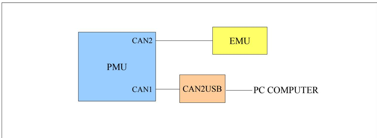
Next, set the correct CAN BUS speed. In this example we use 500kbps and termination on both devices. Remember to use twisted pair cables to connect any CAN BUS devices!
