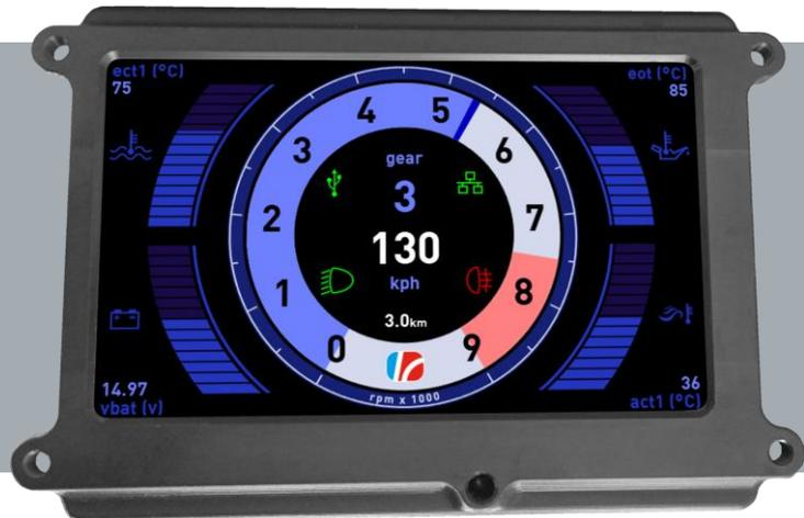
The D4 is a 4.3" Full Colour Sunlight readable WVGA display with 6 general purpose analogue inputs for sensors and 4 switch inputs. 2 flexible CAN2.0B ports, RS232, twin Ethernet ports and real time maths operations allow it to be used as a fully featured central hub for a single connection point. The D4 can log all channels (physical, CAN and maths) to USB at individually configured logging rates or alternatively stream the logged data from LR ECUs (F88, F90, etc).
