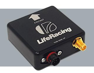
The Life Racing GPS-A10 is a compact low mass unit capable of tracking vehicle speed by GPS position at 10Hz. The unit features a built-in 3-axis accelerometer for measuring lateral, longitudinal and vertical acceleration. The module connects to any device via the CAN network.
