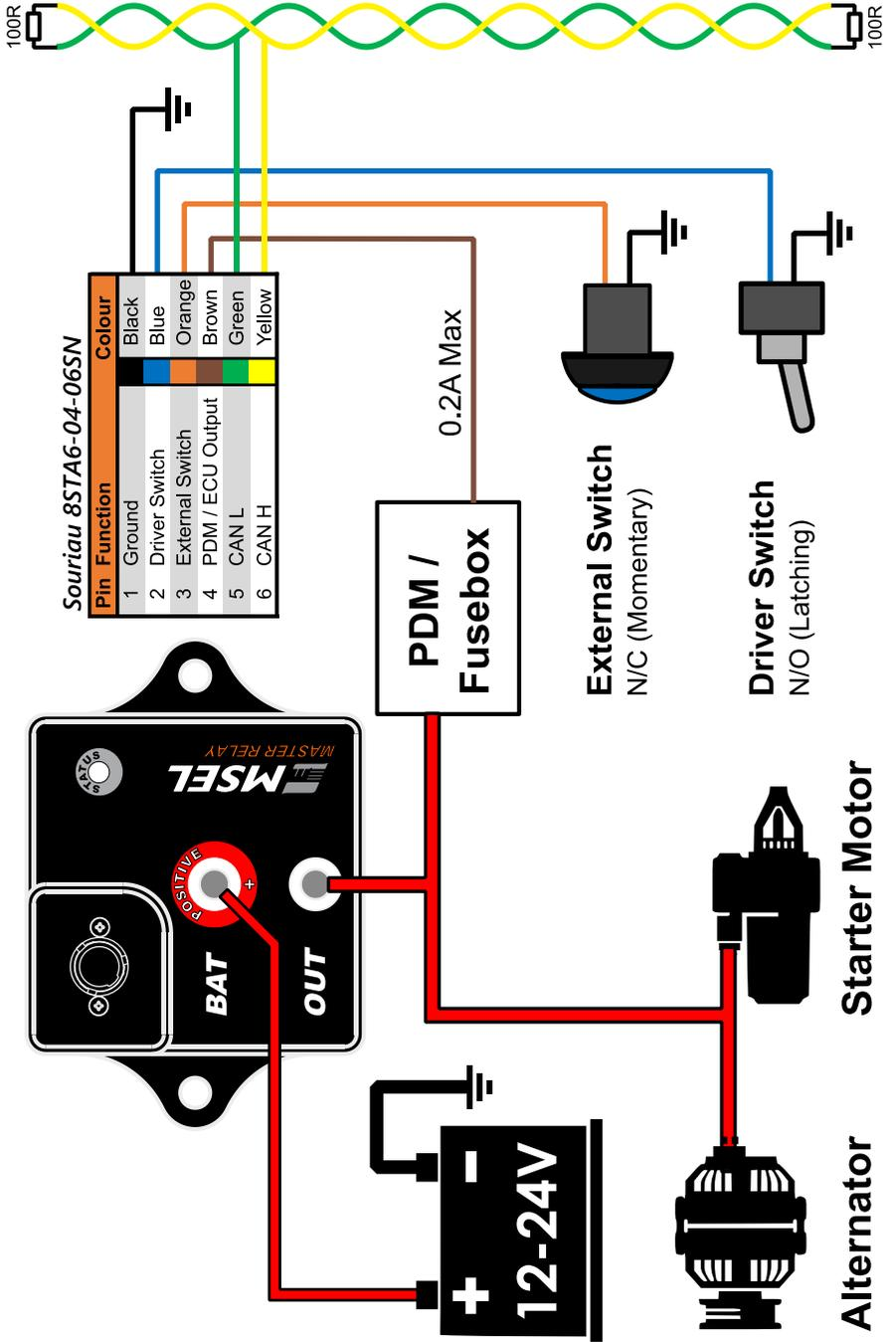
Figure 1: Connection Diagram
