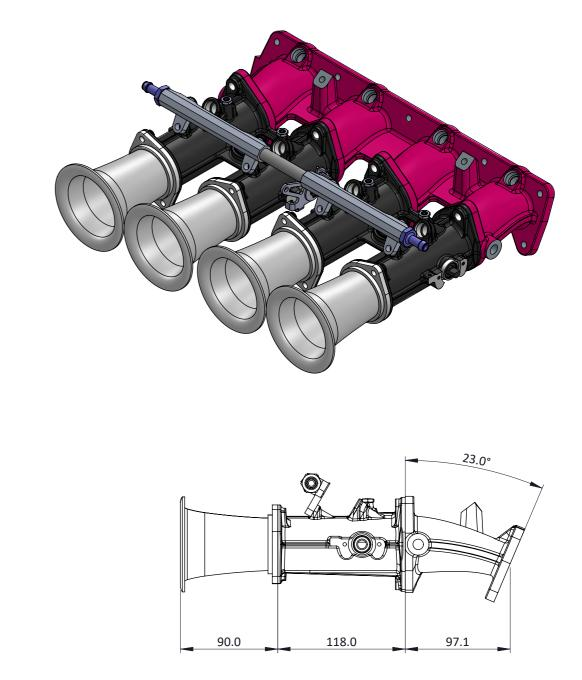
A kit for the Peugeot/Citroen 2.0 engine - EW10 J4 - as used in the 206 GTi which contains an inlet manifold, a pair of TB45's, fuel rail and 90mm long airhorns. Curved to miss the power steeering system. Also fits the EW10J4s (GTI180 & RC) although porting will be required and there is no provision for the inlet manifold oil take-offs.
