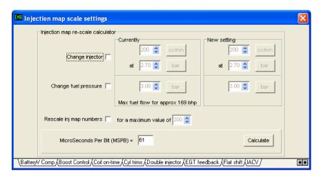
To change the MSPB value, select the "Injector Scaling" option from the "Additional Maps" menu. Simply change the MSPB value, close the window and program the map. It is not necessary to click "Calculate."
