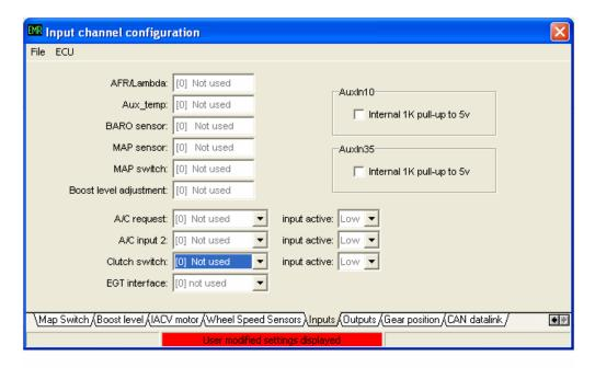
**Input channel configuration:** This page is used to assign ECU pins for various different input functions. Check that AFR and MAP sensor inputs etc are correctly configured if used on your engine configuration.
