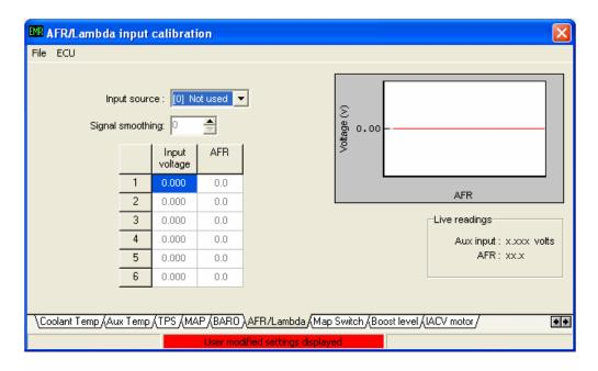
**AFR / Lambda input calibration:** This page is used to provide the respective calibration curve for when a narrow or wide band Lambda sensor is used.
