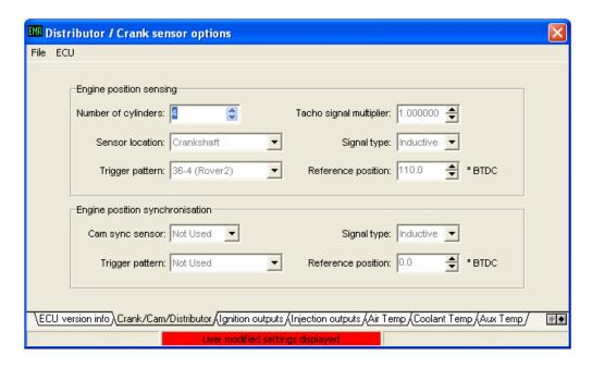
**Distributor / Crank sensor options:** Check to ensure that the parameters set match the physical configuration of your engine.
