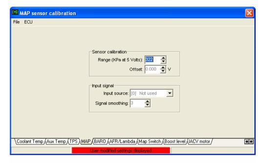
**MAP** sensor calibration: This page will be utilised when using a MAP sensor and should be configured appropriately to suit the range of the MAP sensor fitted.
