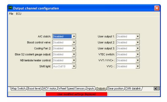
**Output channel configuration:** This page is used to assign ECU pins for various different output functions. Check that Boost valve's and VVT outputs etc are correctly configured if used on your engine configuration.
