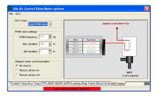
**Idle Air Control Valve Motor options:** For engine configurations using an IACV the control parameters for the valve should be set using this page.
