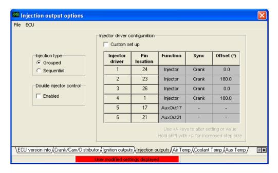
**Injection output options:** Check to ensure that the parameters set match the physical configuration of your engine. Note: Sequential injector operation can only be used where a CAM phase sensor is fitted and connected.
