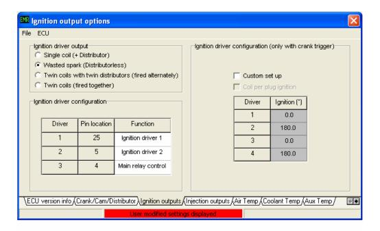
**Ignition output options:** It is important to ensure that the ECU is configured correctly for the type of ignition system in use on your engine. This is particularly important for cars with Coil on Plug (COP) ignition systems as damage can occur to the coils and/or the ECU if incorrectly configured. **Ensure coils are disconnected during modifications to the "Ignition output options" page and update the ECU configuration after completing any changes.**
