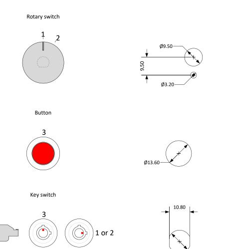
Key/ button switch position 3 overrides rotary switch.
