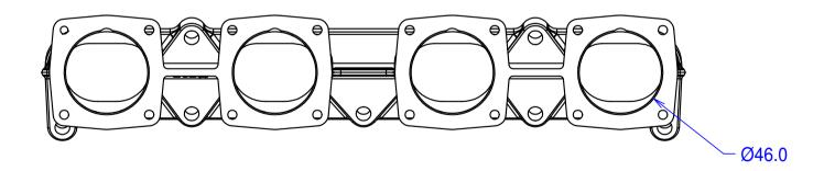
Flanges for Jenvey SF throttle bodies. May be ported up to 50mm. O ring seal to cylinder head Additional material to allow matching to ported cylinder heads Undrilled bosses on underside for idle air / vacumn take off / etc
