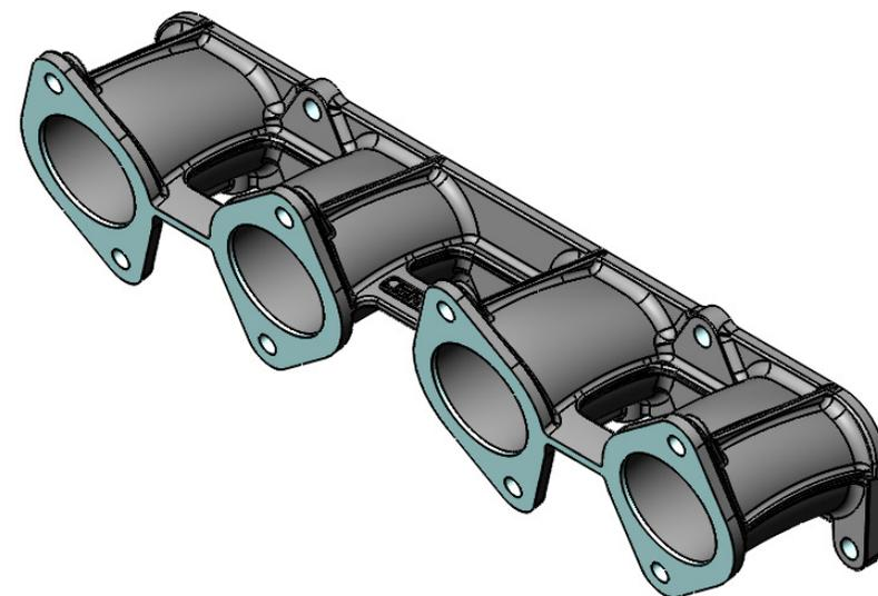
ADDITIONAL MATERIAL TO ALLOW MATCHING TO CYLINDER HEADS.
