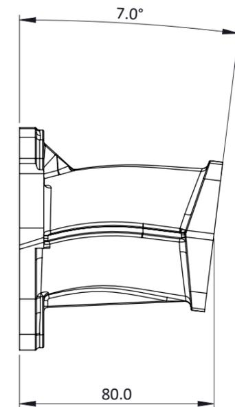
MAY BE PORTED OUT TO 52MM AT INLET FLANGE AND PROPORTIONALLY AT HEAD FLANGE.
