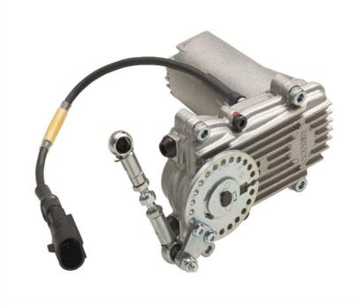
The ETA2 consists of a DC Motor with reduction gearing and is available as standard with a large range of actuating levers and return springs. It can be driven in either direction and includes adjustable end stops. An adjustable limp home spring module is also available. External throttle position sensors are required.
