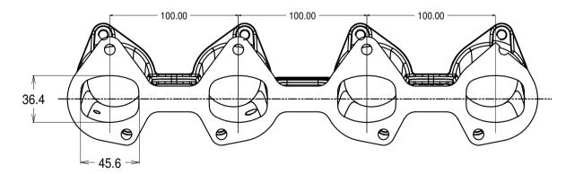
Flanges for Jenvey twin (TB, TH, TS) throttle bodies. May be ported up to 50mm. Additional material to allow matching to ported cylinder heads. Undrilled bosses on underside for idle air / vacumn take off / etc.
