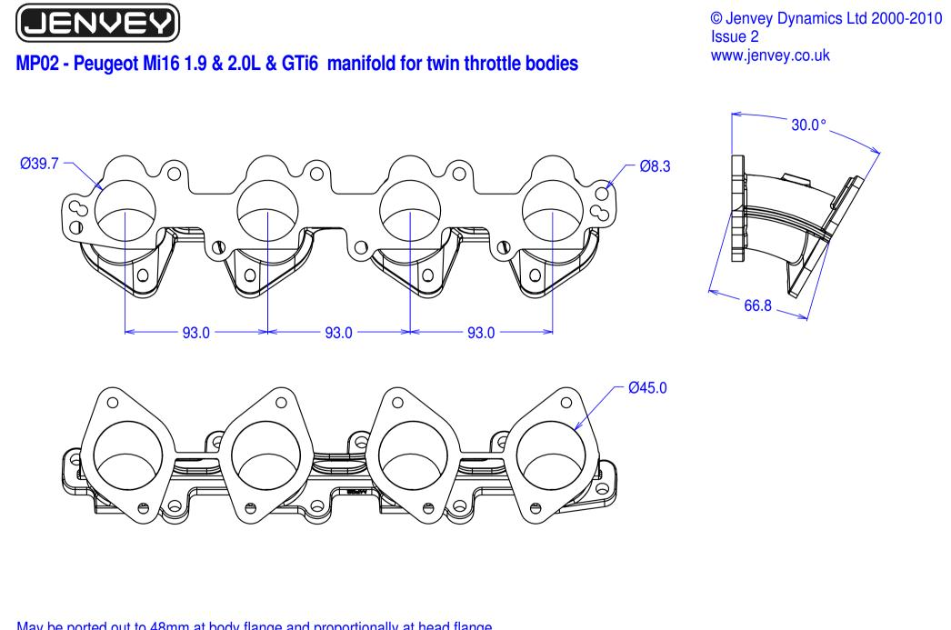
May be ported out to 48mm at body flange and proportionally at head flange. Two bosses on top-side for vacuum tappings.
