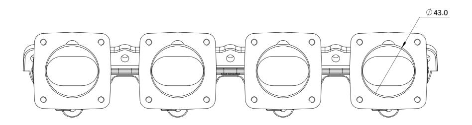
For Jenvey ST throttle bodies or SF with spindle mods. May be ported out to 45mm at body flange and proportionally at head flange. 2 bosses at ends and 4 on underside for vacuum tappings.
