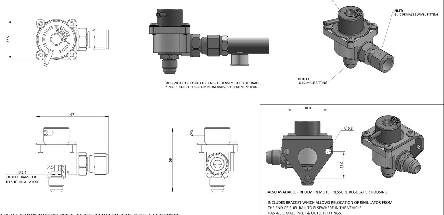
A BILLET ALUMINIUM FUEL PRESSURE REGULATOR HOUSING WITH -6 JIC FITTINGS. THE 9.4mm RELATES TO THE HOLE DIAMETER REQUIRED TO SUIT THE 'O'RING ON THE REGULATOR. COMPATIBLE WITH ALL PRESSURE REGUALTORS SOLD BY JENVEY. \* REGULATOR SHOWN SOLD SEPERATELY.
