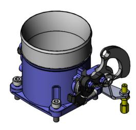
The SFGT throttle body is primarily designed for turbo- or super-charged applications and has a spigot inlet which will accept hose directly from an intercooler, turbo or air filter. It fits directly to the Jenvey 70mm turbo plenum and includes porting and mountings for an idle control valve. Adapters are available for the Mitsubushi Evo8 IC valve.
