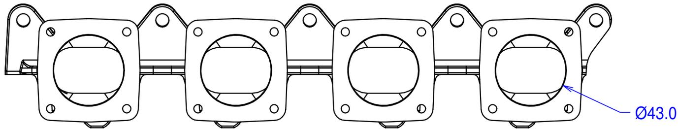
Flanges for Jenvey SF throttle bodies. May be ported out to 46mm at body flange and proportionally at head flange.
