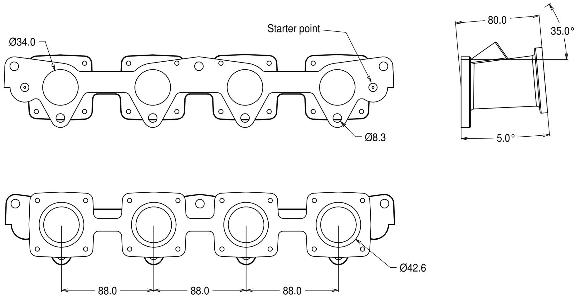
Flanges for Jenvey SF throttle bodies. May be ported out to 46mm at body flange and proportionally at head flange.
