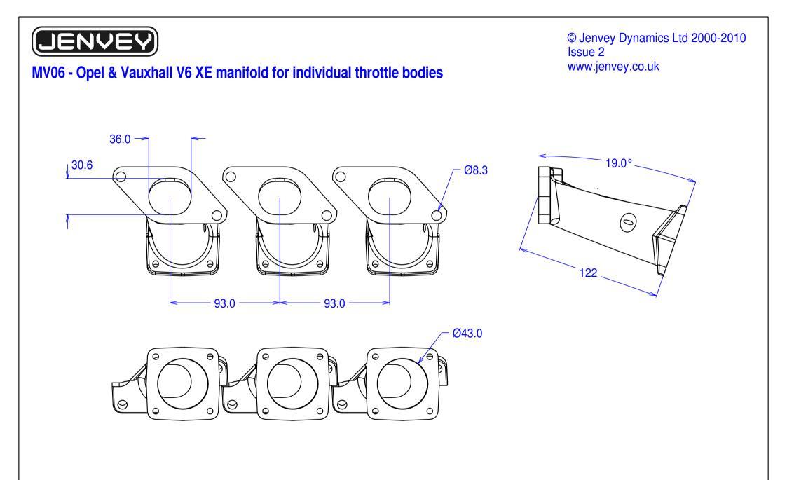
Flanges for Jenvey SF throttle bodies. May be ported out to 46mm at body flange and proportionally at head flange. Bosses on top-side for vacuum tappings.
