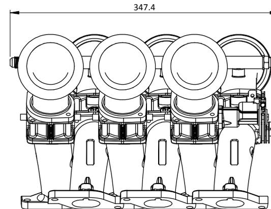
A kit for the Opel/Vauxhall V6XE which contains six stub inlet manifolds, six SFS42 throttle bodies, linkage, a fuel rail for Pico (short) injectors and 42mm curved airhorns. Fits the RWD Omega and will also fit an Astra or Vectra with a little work. The engine was used in the Omega and the Vectra.
