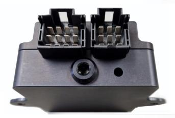
The AWD Unit will come pre loaded with a base calibration that has default values which simulate an OEM Haldex unit. Use Syvecs Scal software to adjust
