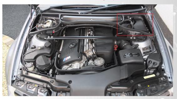
3.) You will then find the engine DME with 5 connectors coming out of it. Unplug these and remove the OEM DME
