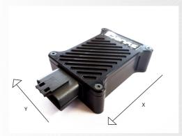
In applications where heavy vibrations are present due to solid engine mounts etc, it is advised to mount the GPS using some rubber washers to absorb some of the vibrations.
