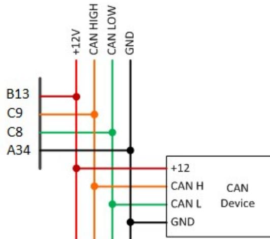
**NOTE:** CAN Wires must be kept as a twisted pair.
