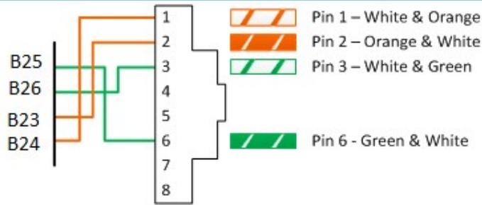
Figure 0-2 RJ45 Wiring
