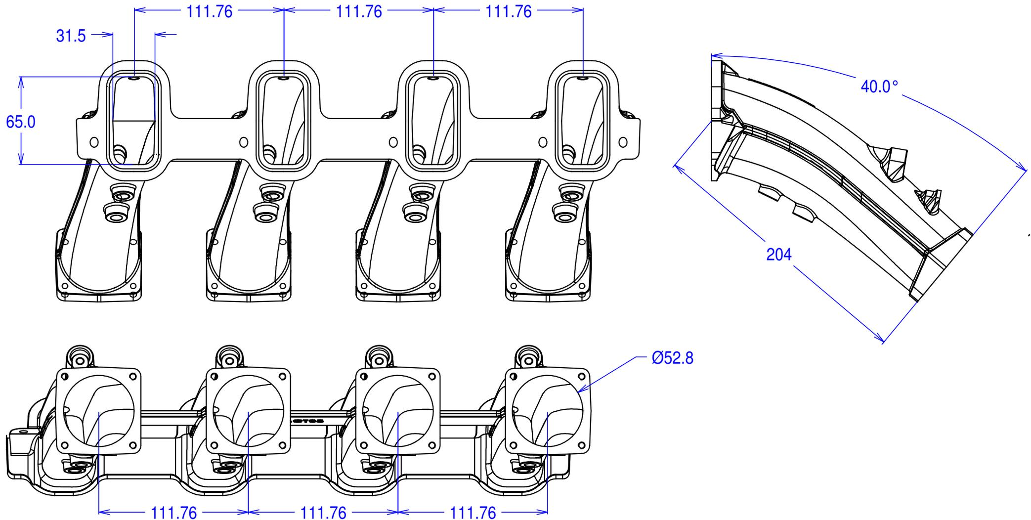
Flanges for Jenvey SFD throttle bodies. Sufficient metal to allow port machining.
