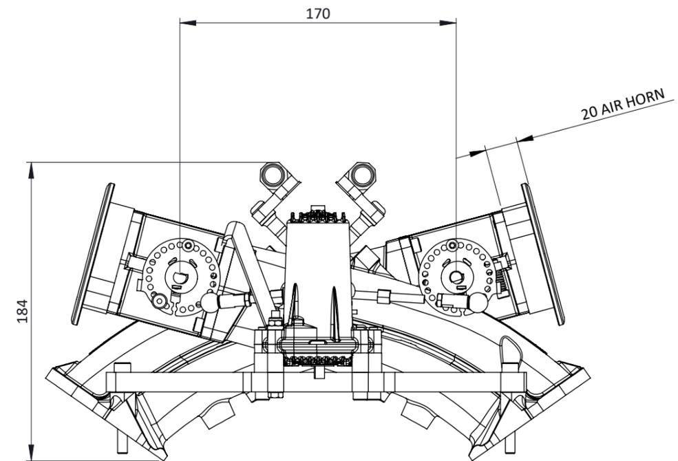
Flanges for Jenvey SFD throttle bodies. Sufficient metal to allow for port machining, including 'Cathedral' shape.
