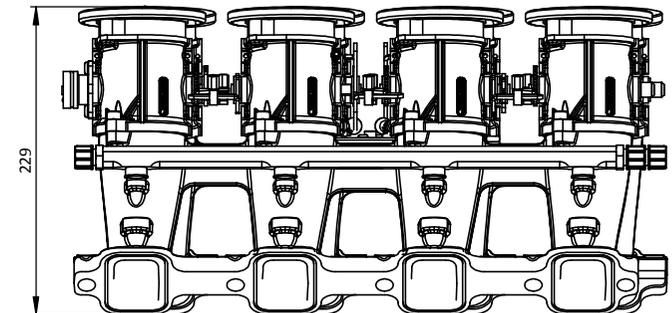
THE JENVEY CHEVROLET LS7 ITB DOWNDRAFT THROTTLE BODY KIT INCLUDES EIGHT SSD60/45/0, Ø57 BUTTERFLY, THROTTLE BODIES WITH CLV6 LS DOWNDRAFT LINKAGE KIT, TWO EFI INLET MANIFOLDS, TWO FUEL RAILS AND EIGHT 20MM LONG BILLET AIRHORNS DESIGNED SPECIFICALLY FOR MOTORSPORT APPLICATIONS OFFERING EXCEPTIONAL PERFORMANCE LIGHTNESS RELIABILITY AND LOOKS. USING OUR MODULAR COMPONENTS OFFERS HUGE OPPORTUNITY FOR BESPOKING TO MATCH YOUR APPLICATION
