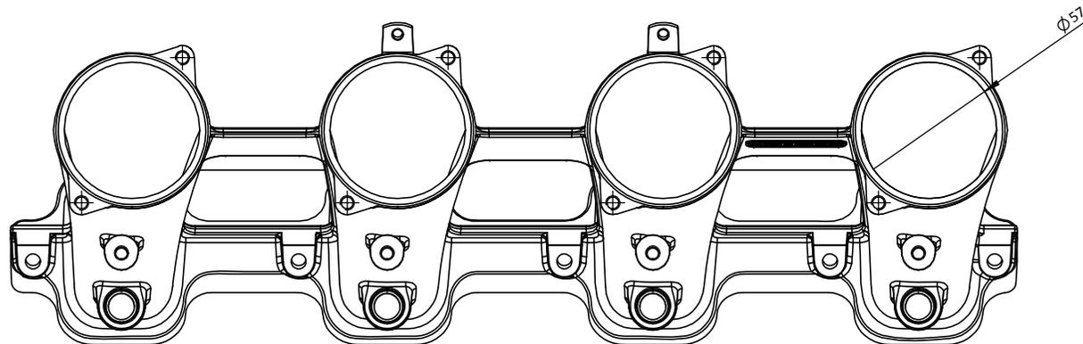
FLANGES FOR JENVEY SSD THROTTLE BODIES. SUFFICIENT METAL TO ALLOW PORT MACHINING.
