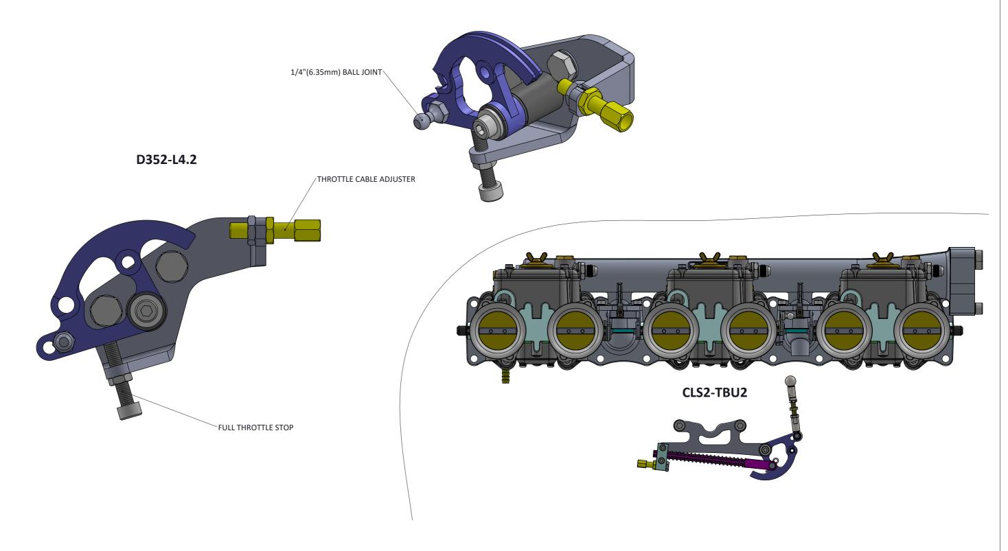
CLJ-4.2RH - ACCELERATOR LINKAGE KIT TO SUIT THE RH DRIVE JAGUAR E-TYPE SERIES 1-2, WITH 4.2 ENGINES, INCLUDES THE FOLLOWING PARTS:
