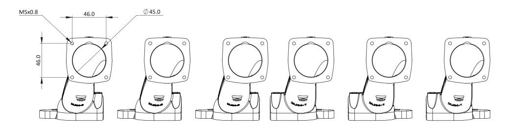
FLANGES FOR JENVEY SINGLE (SF, SFS) THROTTLE BODIES. MAY BE PORTED UP TO 48MM WITH SUFFICIENT MATERIAL TO ALLOW FOR MATCHING TO PORTED CYLINDER HEADS. UNDRILLED BOSSES ON THE UNDERSIDE OF THE MANIFOLD FOR IDLE AIR/ VACUUM TAKE-OFF ETC.
