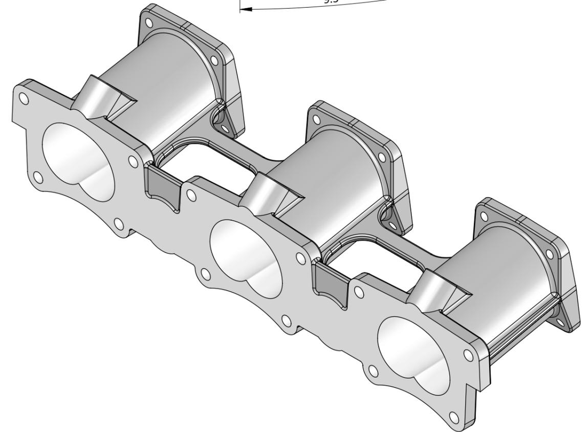
MAY BE PORTED OUT TO 50MM AT BODY FLANGE AND PROPORTIONALLY AT HEAD FLANGE.
