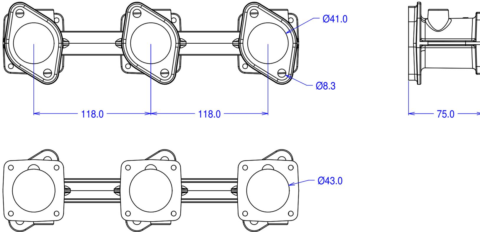
May be ported out to 46mm at body flange and proportionally at head flange.
