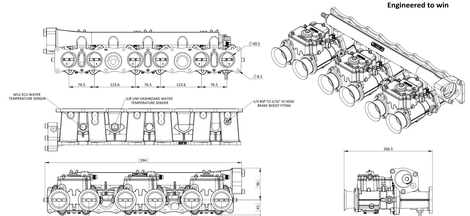
The Jenvey Jaguar XK6 manifold has been designed to suit both the E-Type Series 1 3.8L & 4.2L engines and the Series 2 4.2L engine, With inlet flanges to suit Jenvey DCOE Heritage and standard throttle bodies.
