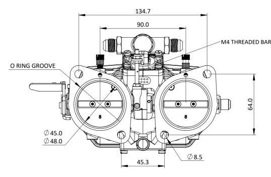
The Heritage body is designed with major dimensions identical to twin vertical carburettors from Weber, Dellorto, Solex etc. The fuel rail is integrated within the body lid, supplied with Bosch injectors.
