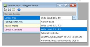
To check the oxygen sensor, start the engine, wait when the sensor heats up, and observe logging channel *Lambda*
