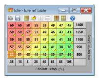
This tables defines the engine rpm when on idle as a function of engine coolant temperature. In addition to air control the idle RPM is controlled in closed loop using **Idle / Ignition control**
