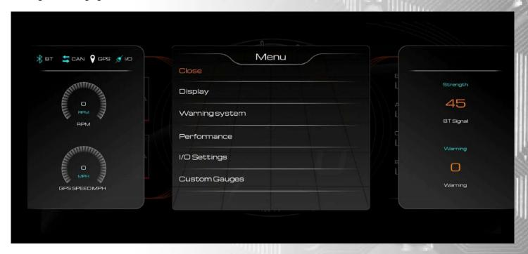
In the example above BT CAN and I/O indicating blue is showing a good connection. GPS shows white in this example as not locked onto GPS satellites. Yellow would indicate a weak signal.
